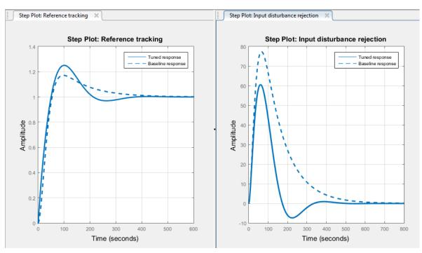
Change the design focus to favor disturbance rejection. In the  $\bigcirc$  **Options** dialog box, in the **Focus** menu, select Input disturbance rejection.
