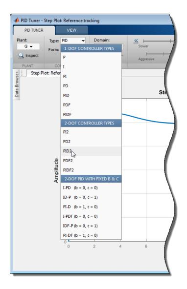
The following tables summarize the available PID controller types. For more information about these controller types, see "PID Controller Types for Tuning".
