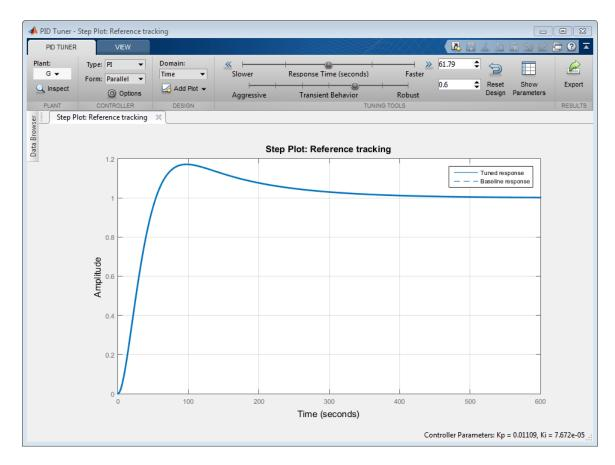
Add a step response plot of the input disturbance rejection. Select  $\mathbf{Add}$   $\mathbf{Plot} > \mathbf{Input}$   $\mathbf{Disturbance}$   $\mathbf{Rejection}$ .
