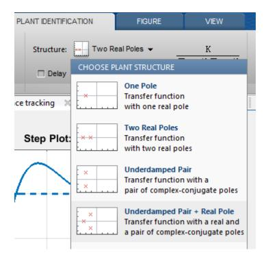
For any chosen structure you can optionally add a delay, a zero and/or an integrator element using the corresponding checkboxes. The model transfer function configured by these choices is displayed next to the **Structure** menu.
