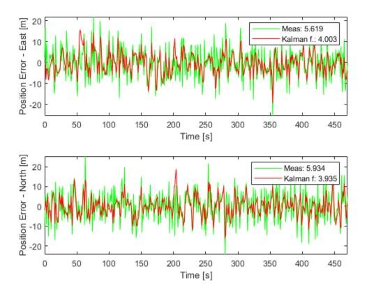
The plot legends show the position measurement and estimation error ( $||x_e - \hat{x}_e||_1$  and  $||x_n - \hat{x}_n||_1$ ) normalized by the number of data points. The Kalman filter estimates have about 25% percent less error than the raw measurements.
