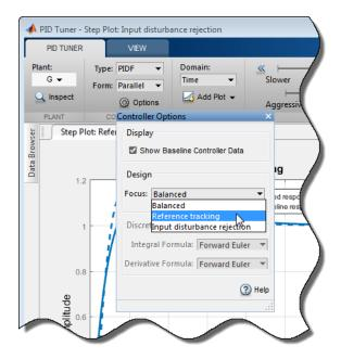
**PID Tuner** automatically retunes the controller coefficients with a focus on reference-tracking performance.
