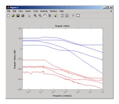
The reduction error is small compared to the original system so the reduced order model provides a good approximation of the original model.
