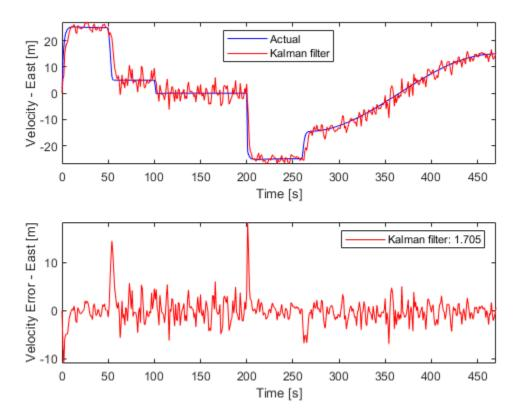
The legend on the error plot shows the east velocity estimation error  $||\dot{x}_e - \dot{x}_e||_1$  normalized by the number of data points.
