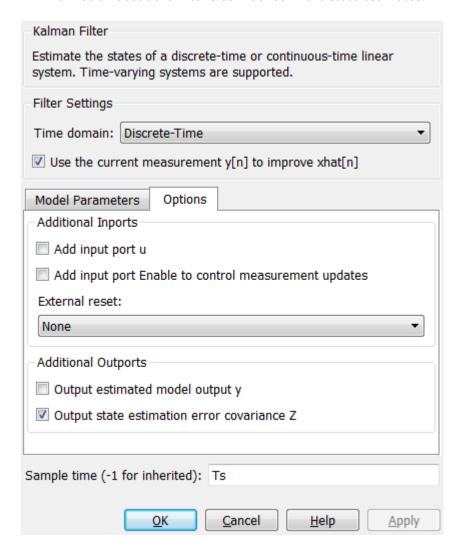
Click **Model Parameters** to specify the plant model and noise characteristics:
