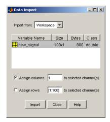
6 Click **Import**. This imports the new signal into the Linear Simulation Tool.
