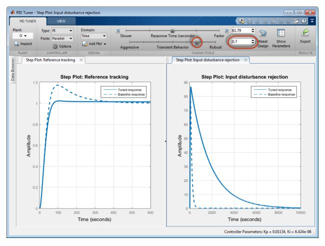
Increasing the transient-behavior coefficient to 0.70 nearly eliminates the overshoot, but results in extremely sluggish disturbance rejection. You can try moving the **Transient behavior** slider until you find a balance between reference tracking and disturbance rejection that is suitable for your application. The effect that changing the slider has on the balance depends on the plant model. For some plant models, the effect is not as large as shown in this example.
