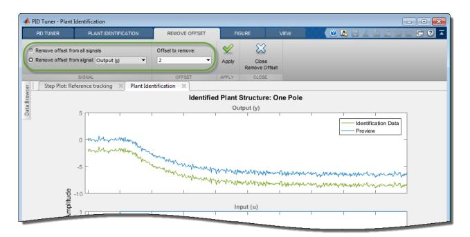
Click Apply to save the change to the signal. Click Close Remove Offset to return to the Plant Identification tab.
