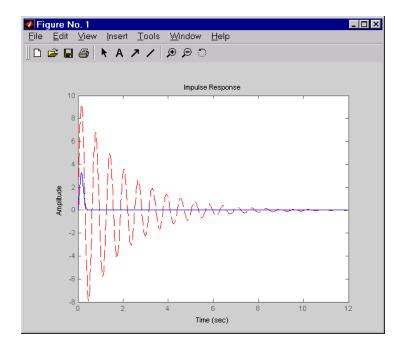
**Comparison of Open- and Closed-Loop Impulse Response**
